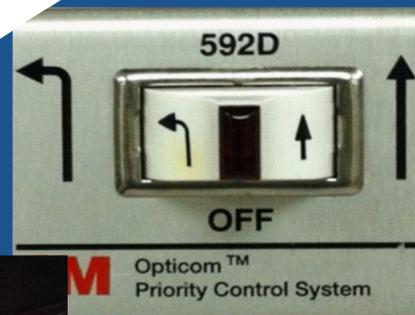
*The Emergency Vehicle operator slides the selector switch to the left to activate preemption. (Sliding to the right extends the green.)*
