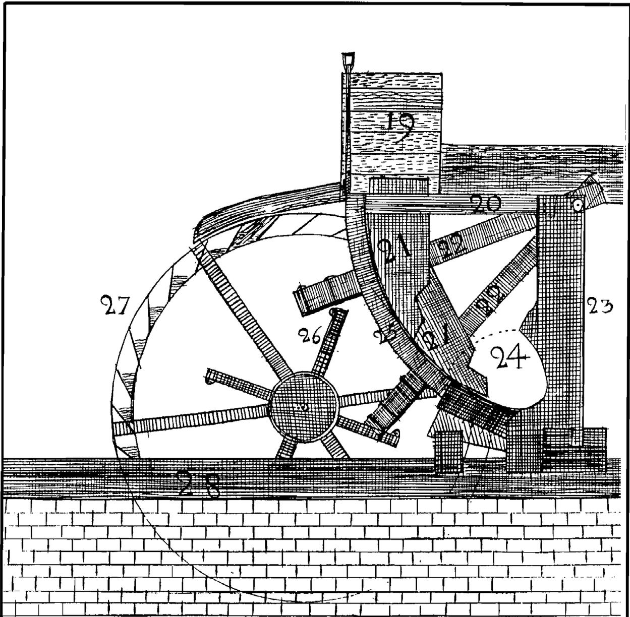
19 Penstock, water-gate and spout of an overshot fulling mill.
