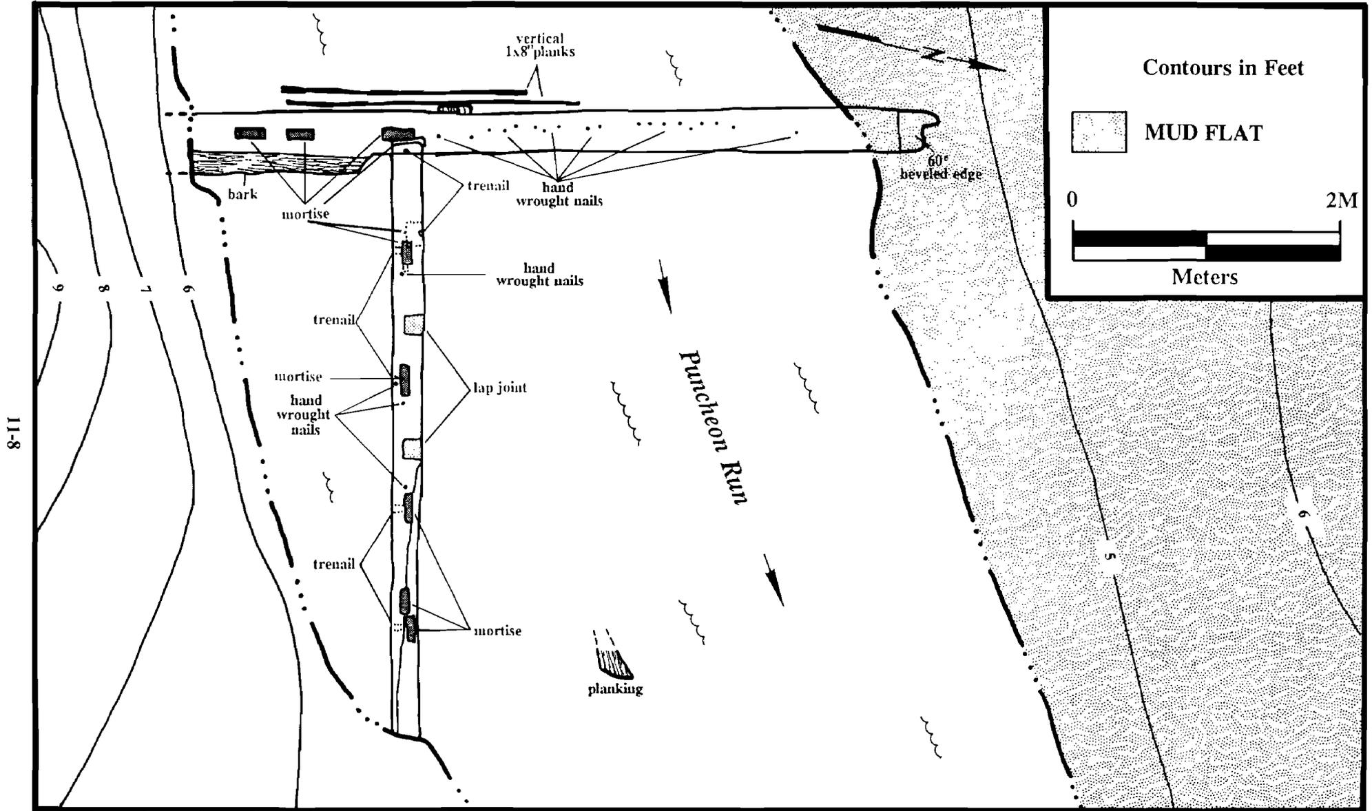
Figure 11.2. Area B, Nixon Mill Site, Detailed Plan of Timber Remains at the Southern End of the Mill Dam.
