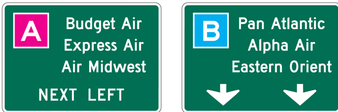
Figure 2D-1. Examples of Color-Coded Destination Guide Signs
