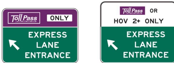
Figure 2G-18. Examples of Guide Signs for Entrances to Priced Managed Lanes
