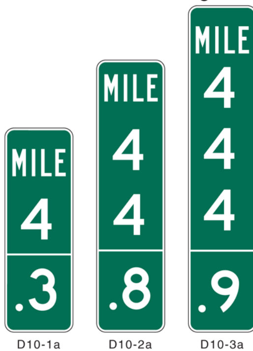
Figure 2H-3. Intermediate Reference Location Signs
