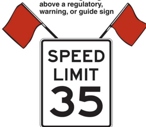
Figure 2A-1. Examples of Enhanced Conspicuity for Signs
