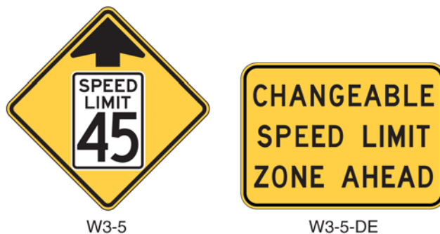
Figure 2C-7. Reduced Speed Limit Ahead Signs (Delaware Revision)
