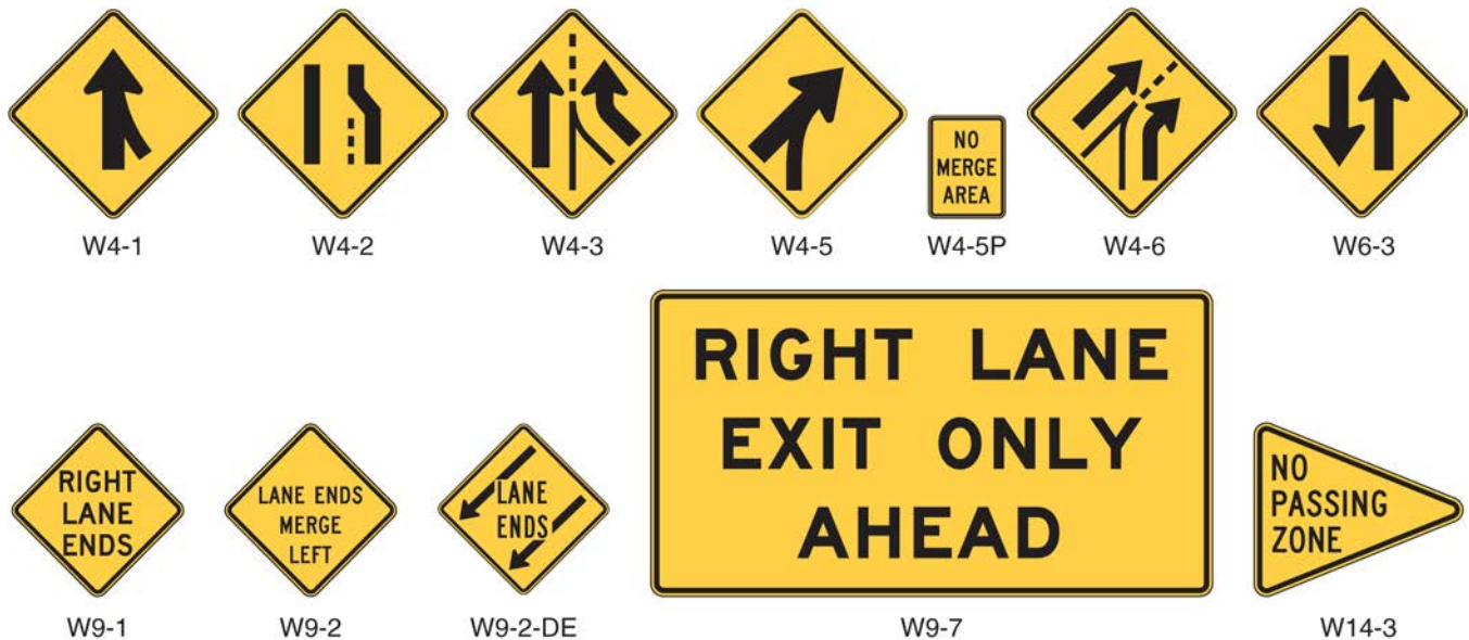
Figure 2C-8. Merging and Passing Signs and Plaques (Delaware Revision)
