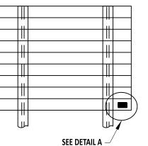
**INSTALL DECAL TO FIRST EXTRUDED** SIGN PANEL JUST BELOW CENTER STIFFNER **RIB APPROXIMATELY 2 TO 3 INCHES FROM RIGHT EDGE OF SIGN PANEL**
