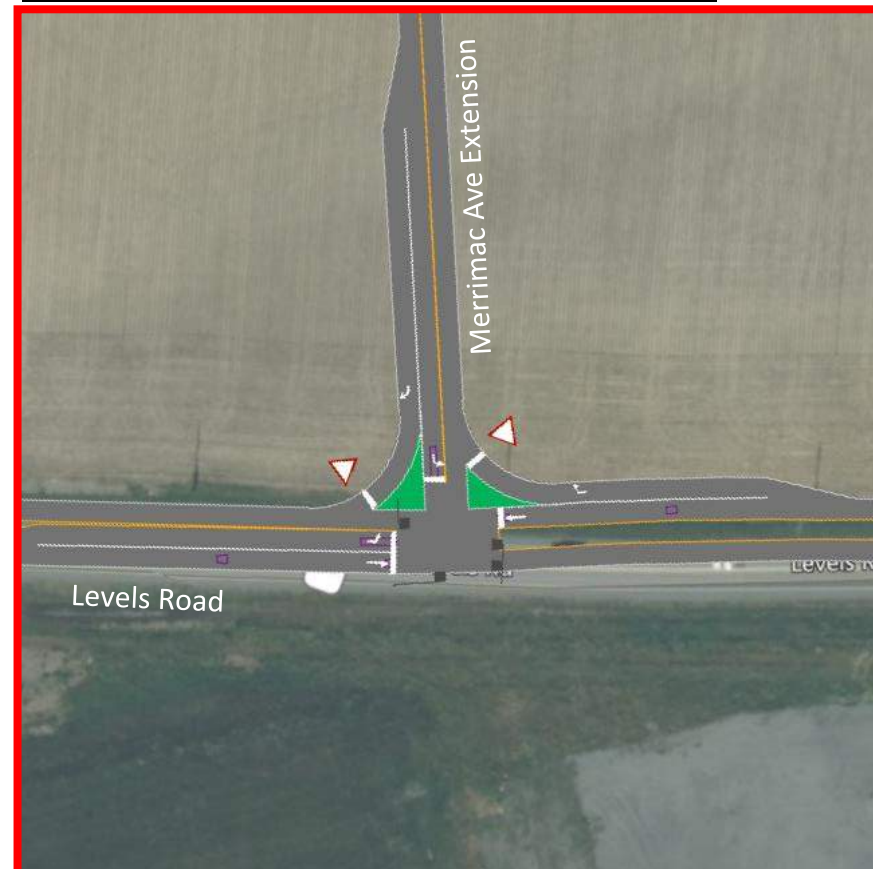
Detail 2 – Install Additional Access Point and Signalize
