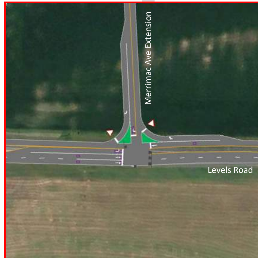
Detail 2 – Install Additional Access Point and Signalize
