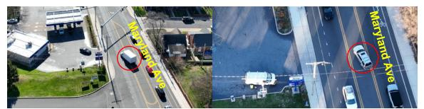
Figure 13: Vehicles using painted median to turn left into the gas station near Robinson Ln / Clayton Dr
