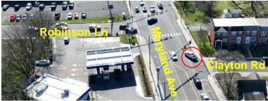
Figure 11: Southbound right-turning motorist made illegal right turn on red arrow and subsequently stopped between Robinson Rd and Clayton Rd without signal head to indicate when to proceed
