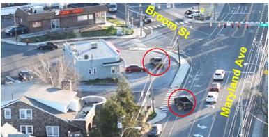
Figure 14: Eastbound left-turning motorists using restaurant parking lot to avoid waiting at red arrow at Broom St
