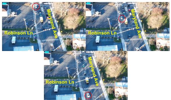
Figure 10: Motorist using right-turn lane and bike lane to pass queued vehicles at Robinson Ln
