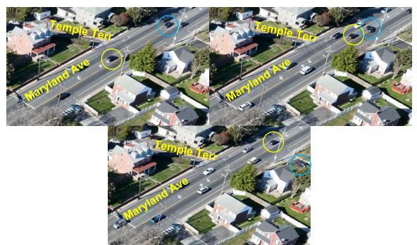
Figure 7: Eastbound motorist (circled in yellow) traveling in two-way left turn lane and successfully navigating around westbound left-turning motorist (circled in blue) waiting in two-way left turn lane for gap (appropriate behavior)
