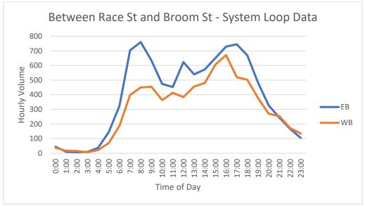
Figure 4: System loop data at Broom St (WB) and Race St (EB)
