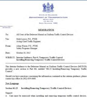
01 Care must be exercised when installing and removing temporary traffic control devices. Installing TTC begins and ends as a mobile operation. Standard:
