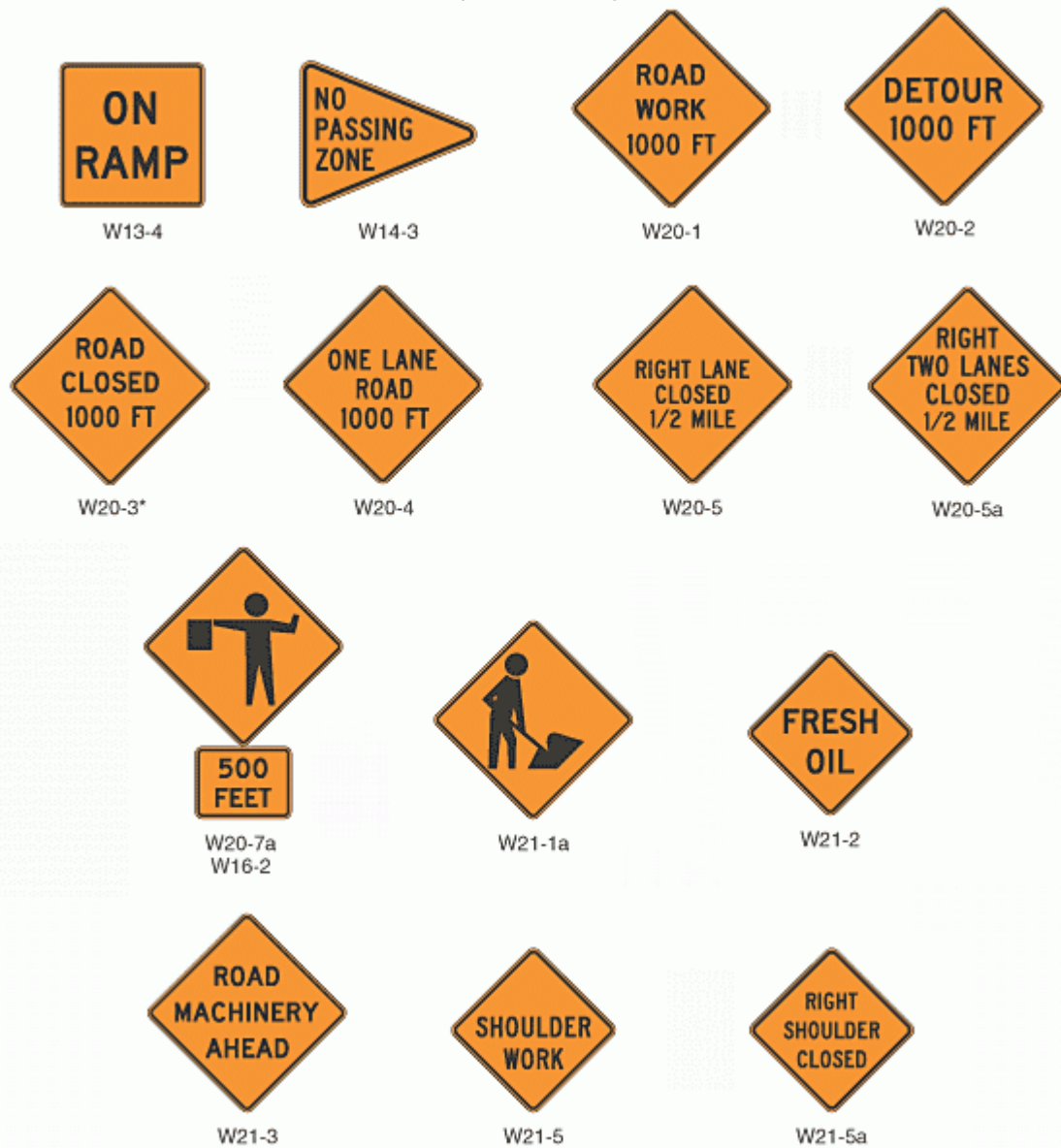
Figure 6F-4. Warning Signs in Temporary Traffic Control Zones (Sheet 3 of 4)
