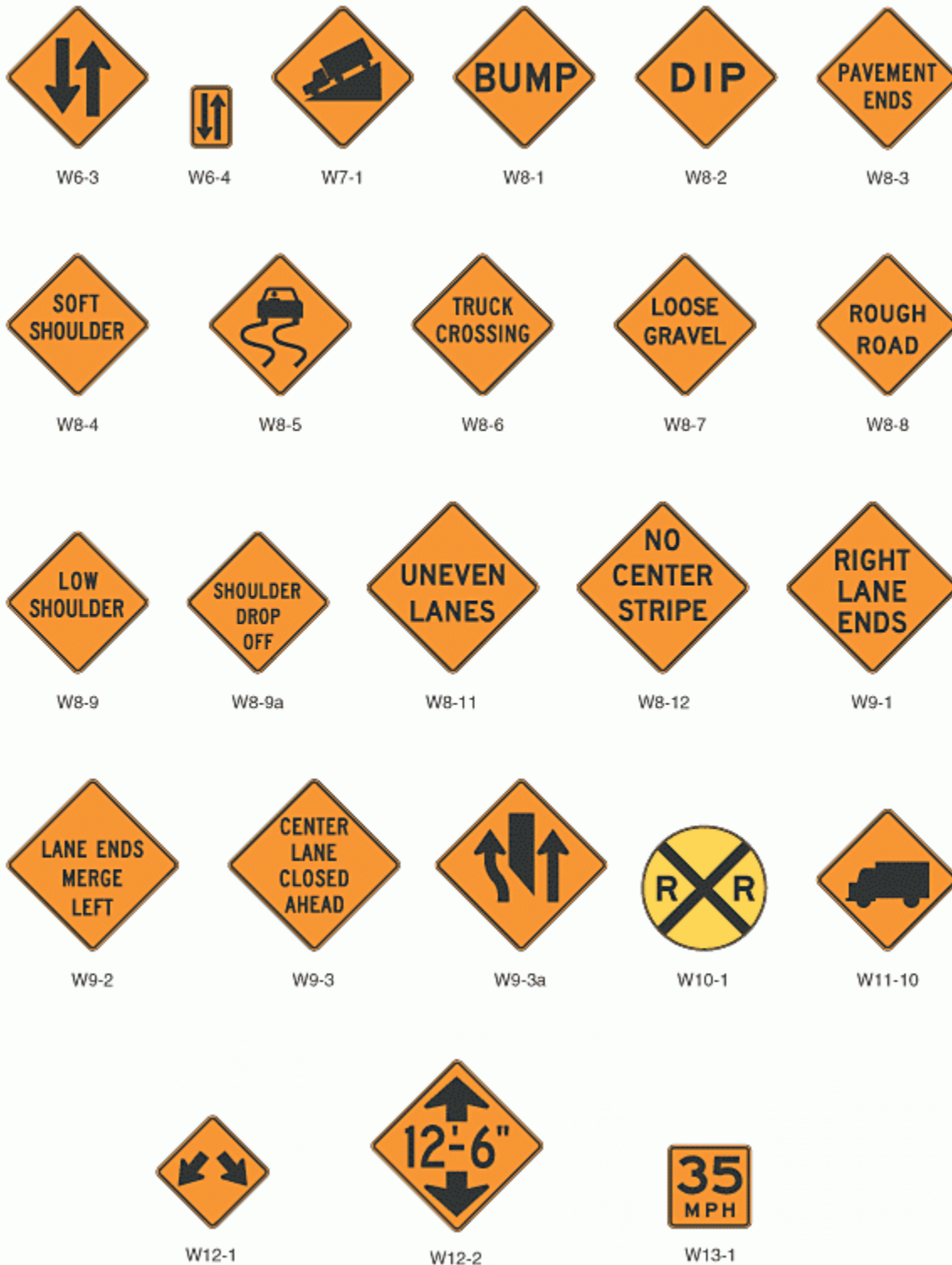
Figure 6F-4. Warning Signs in Temporary Traffic Control Zones (Sheet 2 of 4)
