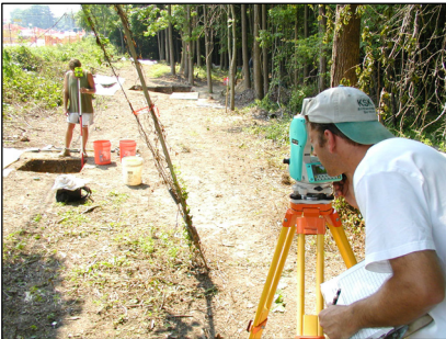
Archaeologists map the locations of the test units with a Total Station laser transit to precisely measure distance and elevation.
