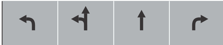
Figure IV-6c. One Left-Turn Lane, One Shared Left/Through Lane, One Through Lane, and One Right-Turn Lane (Split Phasing)
